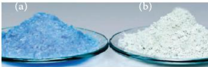
a) Crystalline hydrated salt b) Amorphous anhydrous salt
