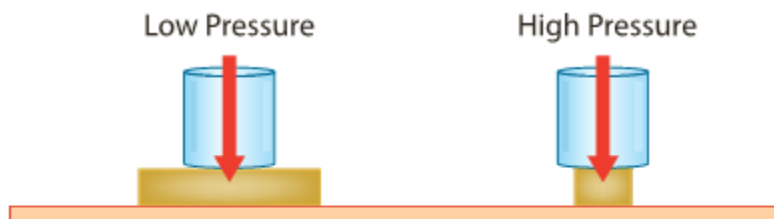
Figure 3.1 Pressure depends on area of application
