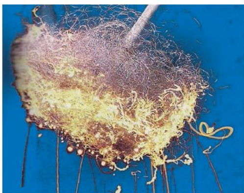
Iron wool (made into thin fibres) burns in oxygen to produce both heat and light energy
